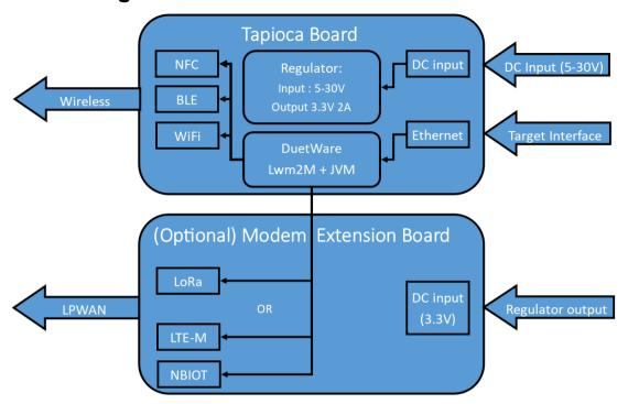
The Tapioca is made up of a standard TapNLink module connected to a Ethernet transceiver. The firmware of the Tapioca gateways is the standard Duetware for TapNLink, TapNPass and Tapioca.
