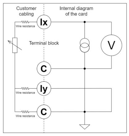
For 3 wire resistance inputs two analog inputs are used:
