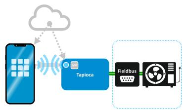
Connect Tapioca directly to sensors with fieldbus (Modbus)
